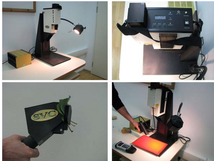
Figure 2: The SVC HR-1024 spectroradiometer
